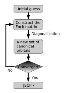
Figure 5.1: The self-consistent field procedure.
