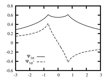
Figure 2.1: Nuclear cusps. Wave functions corresponding to the two lowest eigenvalues of  $H_2$  molecule, along the H–H bond (obtained from a FCI calculation in cc-pVDZ basis).
